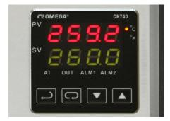
To change or rather to set the welding temperature (lower green shown value) press the appropriate arrow-buttons / below the display. The set point reading starts to flicker. By pressing the button , the shown value will be activated. Now the setpoint is shown as stable value without blinking in the lower display.
