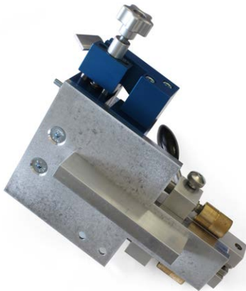
Positioning of clamping holder for vice
