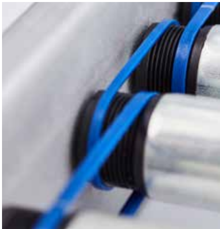
Roller to roller drive
