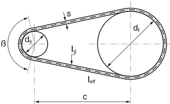
$$l_{eff} = 2c \cdot \sin\left(\frac{\beta}{2}\right) + \frac{\pi}{2} \left[ d_s + d_l + 2s + \frac{(d_l - d_s)(180 - \beta)}{180} \right] \text{ [mm]}$$
