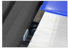
Welding stop for repeatable welds
