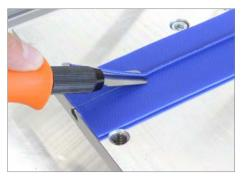
Easy removal of the welding bead with the supplied tool
