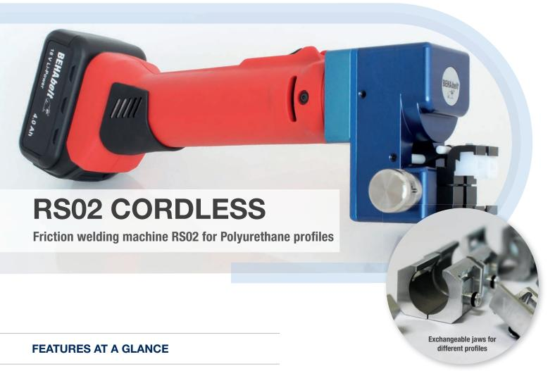
Friction welding machine RS02 for polyurethane profiles eliminates downtime with a perfect splice every time!
