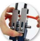
Quick clamp device for inserting the profiles.
