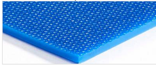
Bottom side: Fabric impression (FI)
