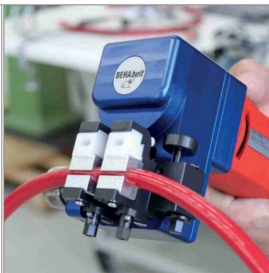
Welding/joining technology for PU and TPE
