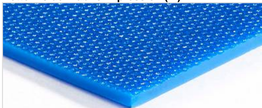
Bottom side: Fabric impression (FI)
