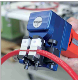
Welding/joining technology for PU and TPE
