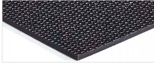
Bottom side: Fabric impression (FI)
