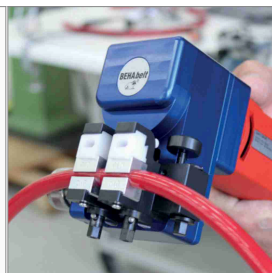
Welding/joining technology for PU and TPE
